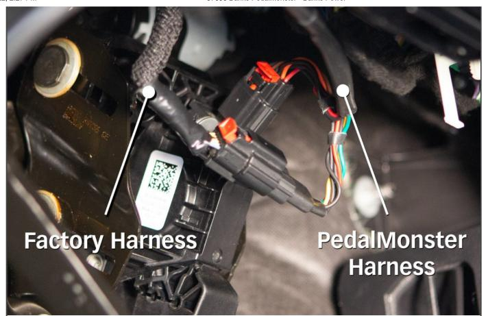
4. Connect the female PedalMonster plug to the accelerator pedal. Connect the male PedalMonster connector to the vehicle's female connector. Ensure both male and female connectors on the PedalMonster module are securely connected to the vehicle's connectors.
